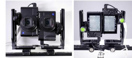
Fig. 4 Top-to-top arrangement of cameras using a pair of vertical posts on a bar
