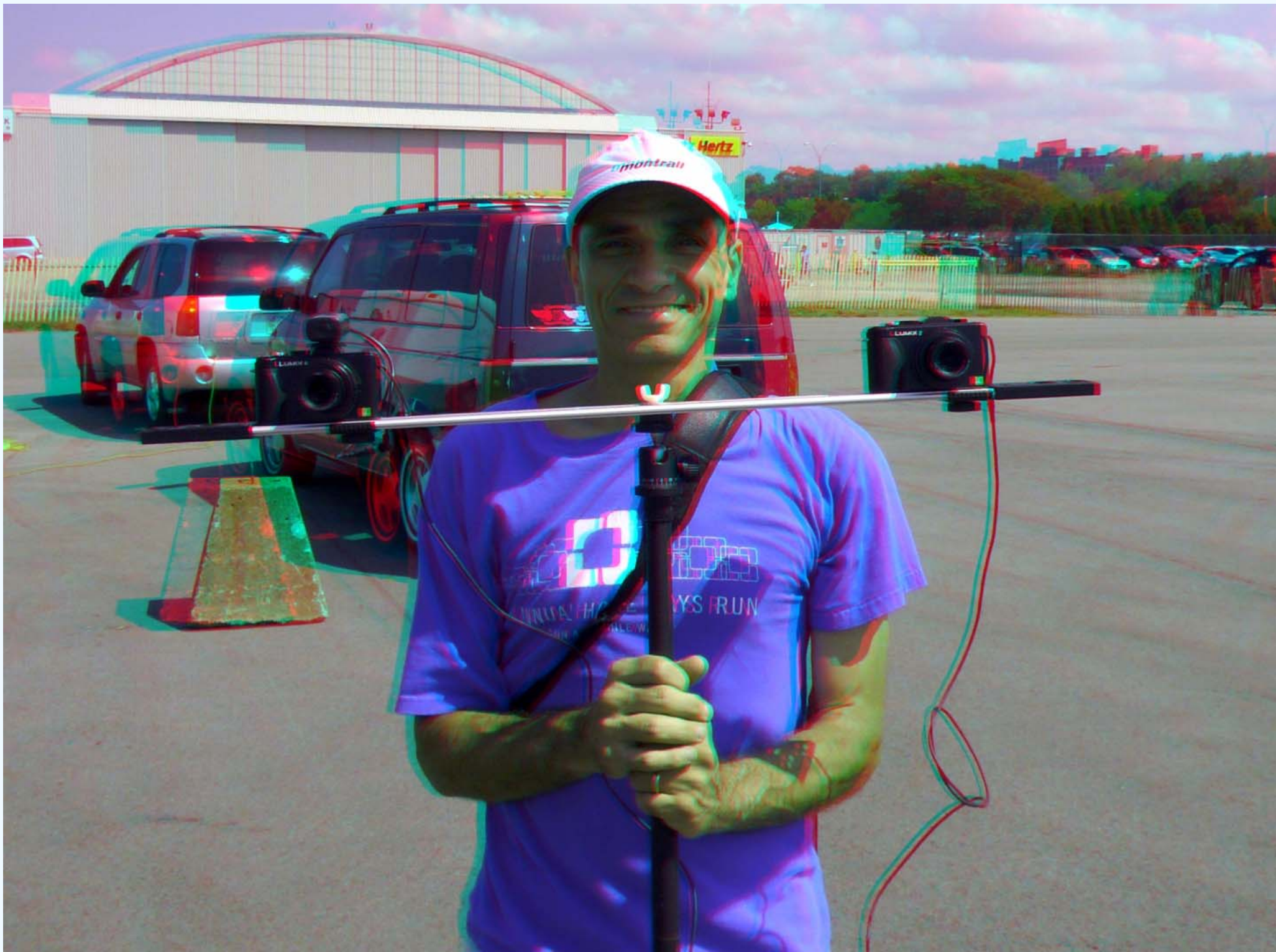
Pole 3D photography with twin Panasonic cameras wired by Ekeren
