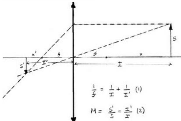
I find myself using the basic lens equation quite a bit so I would like to derive some important formulas. Consider a lens of focal length  $f$ . The object is at distance  $l$  from the lens, while the image is formed at distance  $l'$ . The size of the object is  $s$ , the size of the image is  $s'$ . See the diagram here.
